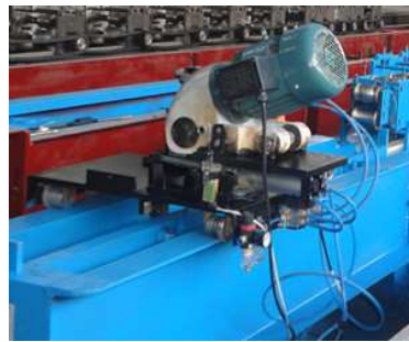
飞锯切割 fly sawing cutting
